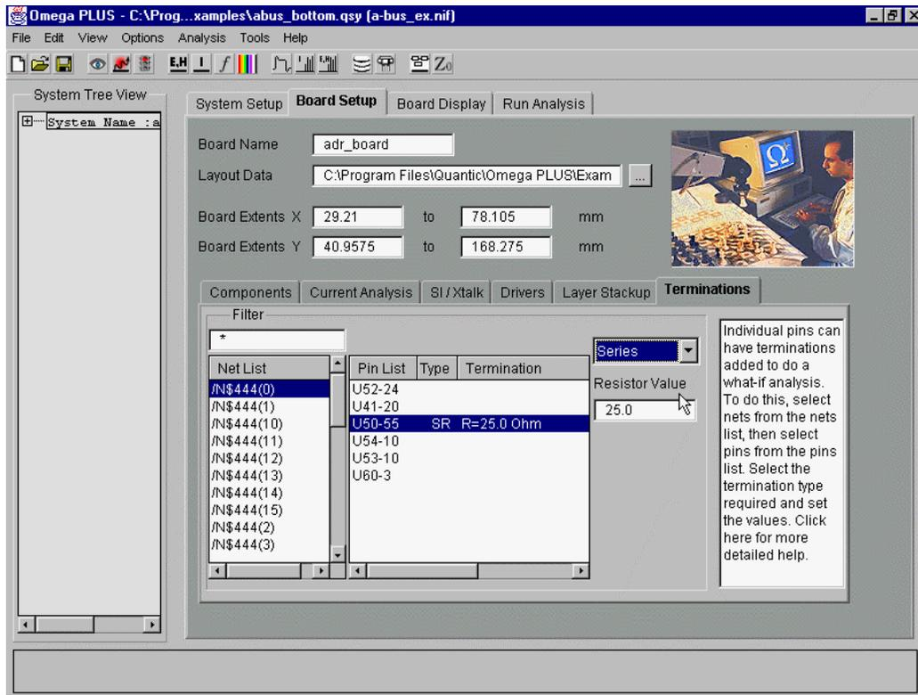
Figure 6. Editing a termination resistor value to suppress emissions.
