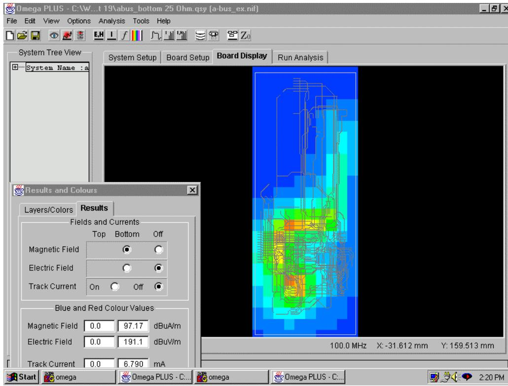
Figure 8. Reduced emissions with 25 Ohm resistor placed in series with the driver pin. Compare with Figure 2.
